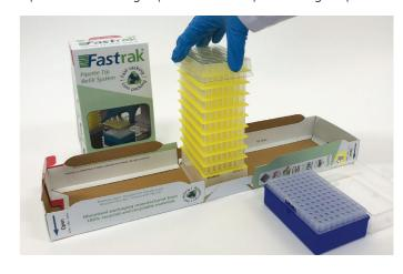
Align the transfer top over a rack and lower refill into position.
