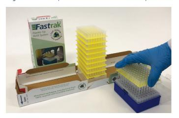
Push down on the transfer top to release the refill plate. Return the transfer top to the *Fastrak* refill stack and close.
